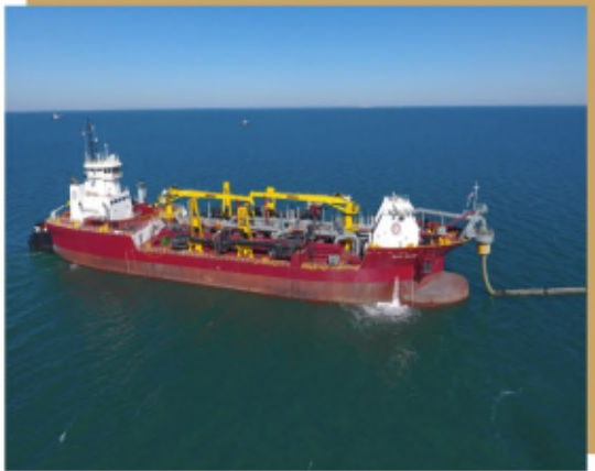
Great Lakes Dredge & Dock – Ellis Island Hopper Dredge – 14,800 cy Eastern Shipyard, FL - $160 M. (Delivered, in service 2018)
