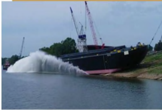
The Dutra Group Two 6,000 CY Split Hull Dump Scows Corn Island Shipyard, IN (1 st scow delivered, in service July 2019)
