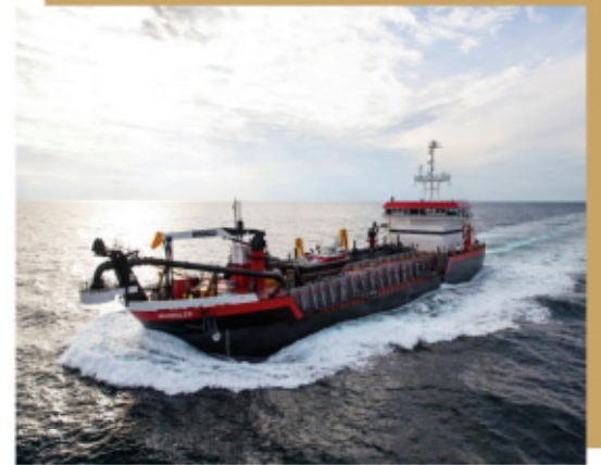
Weeks Marine – Magdalen Hopper Dredge – 8,550 cy Eastern Shipyard, FL - $110 M. (Delivered, in service 2018)
